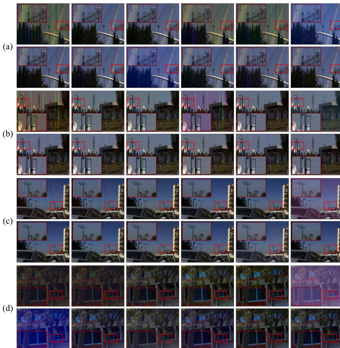
Fig. 6. Denoising results on ICVL dataset with synthetic complex noise. Examples for all the competing methods on band 5, 12 and 20 of the ICVL dataset under 5 complex noise cases are presented respectively. For each group of results, from top to bottom, left to right: Noisy Input, LRTD [18], NMoG [30], LRTDGS [14], FastHyMix [31], SGIDN [23], QRNN3D [32], T3SC [33], and MAC-Net [34], DnRCNN [24], \hat{N} -Net [35], Proposed SLDR.
