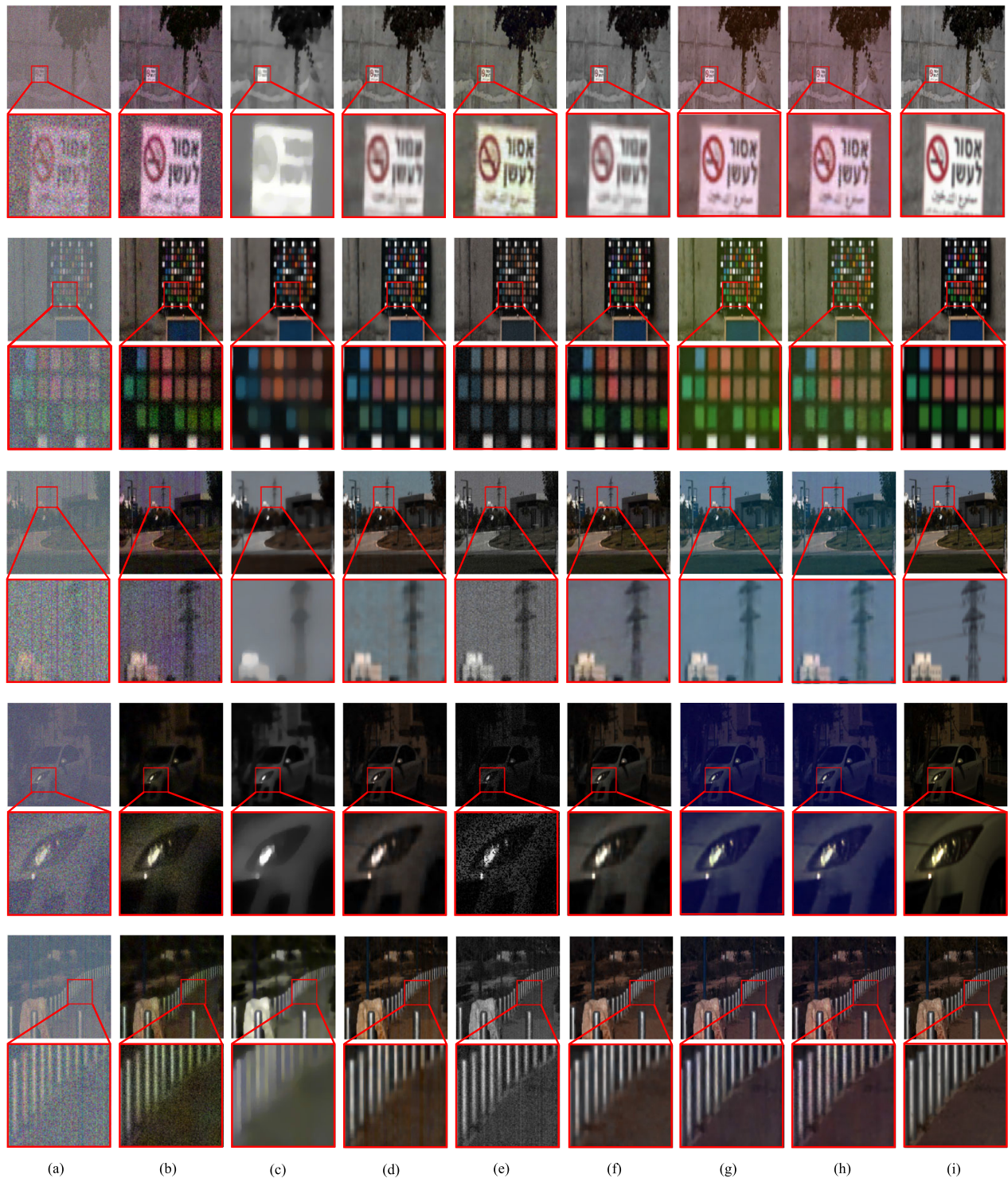
Fig. 8. Simulated complex noise removal results on the ICVL dataset. Examples for all the competing methods on bands 5, 12, and 20 of the ICVL dataset under Cases 2–6 are presented, respectively. Zoomed-in view gives better visualization. (a) Noisy his. (b) LRMR. (c) LRTV. (d) LRTDTV. (e) NMoG. (f) HSID-CNN. (g) QRNN3D. (h) our SQAD. (i) Ground truth.
