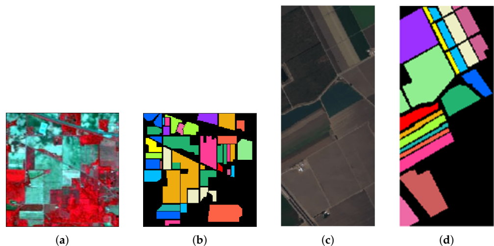
Figure 8. (a) The false color image of the Indian Pines dataset [57], (b) The corresponding ground-truth map. (c) The false color image of the Salinas dataset [22], (d) The corresponding ground-truth map.
